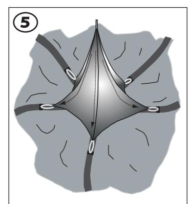
place the cupola fabric over the shaft and snap to the webbing loop along the tunnels. if applicable: place the cupola flag onto cupola shaft.
