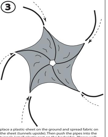
the sheet (tunnels upside). Then push the pipes into the tunnels (small plastic part on the backside). Please walk on fabric without shoes and take care about a clean ground.
