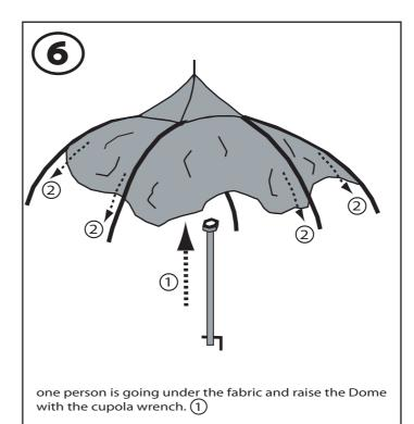
the other person(s) lift and twist the frame legs in a straight position to the center-hub and pulling the fabric down towards the ground. (2)
