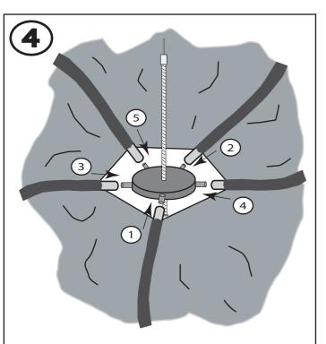
place the cupola hub with the fixed cupola shaft into the center opening of the fabric. (the long part of the shaft on upper side). Then connect the frame legs to the cupola hub. Please mind to do this according to No. 1 - 5. Sliding the fabric inward towards the center opening will ease the legs connection to the hub.
